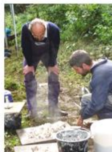
5. Steam rises from slaking lime, at an experimental kiln firing at Whitlingham, 2010.
